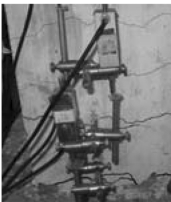
Fig. 3 Typical flexural failure of column specimens
