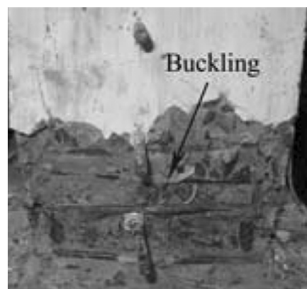
Fig. 3 Typical flexural failure of column specimens
